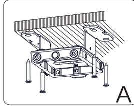
A. Separate the (1) ceiling cover and the (2) Angle Adjuster. Install the ceiling cover to the ceiling. Then, Put in the (4) Decoration cover.
