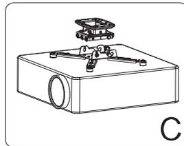
C. Combine the installation arms part to the ceiling fixing parts.
