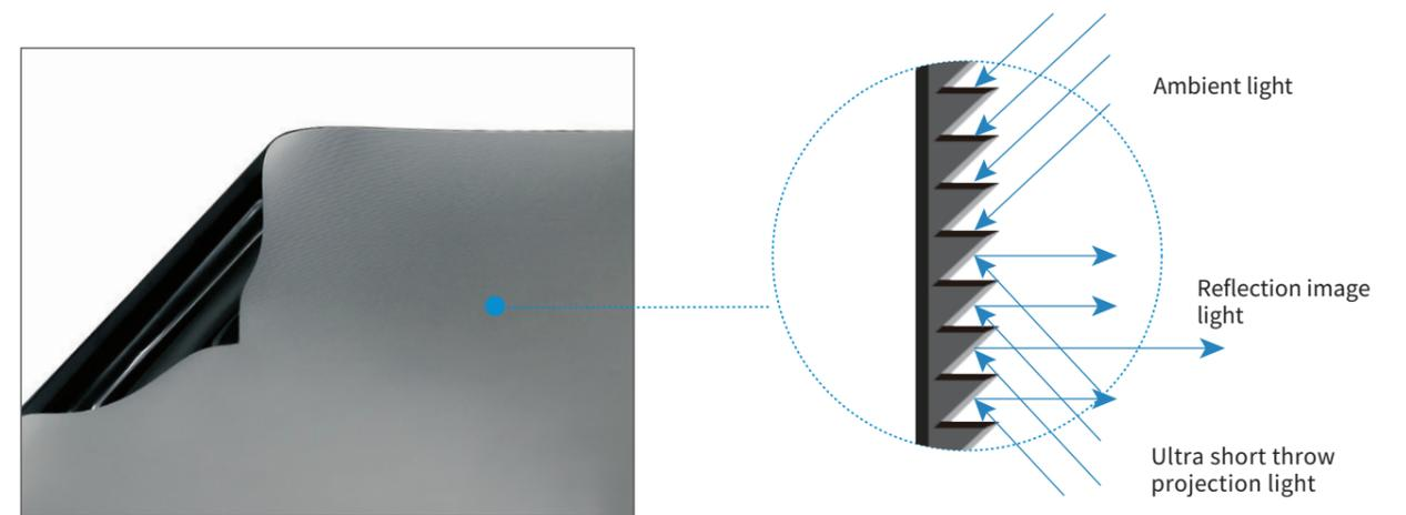
② The screen surface is created using a seaming process. The seams may exhibit a certain degree of curvature due to the tension applied above and below, which does not affect the actual projection and is considered a normal phenomenon.
