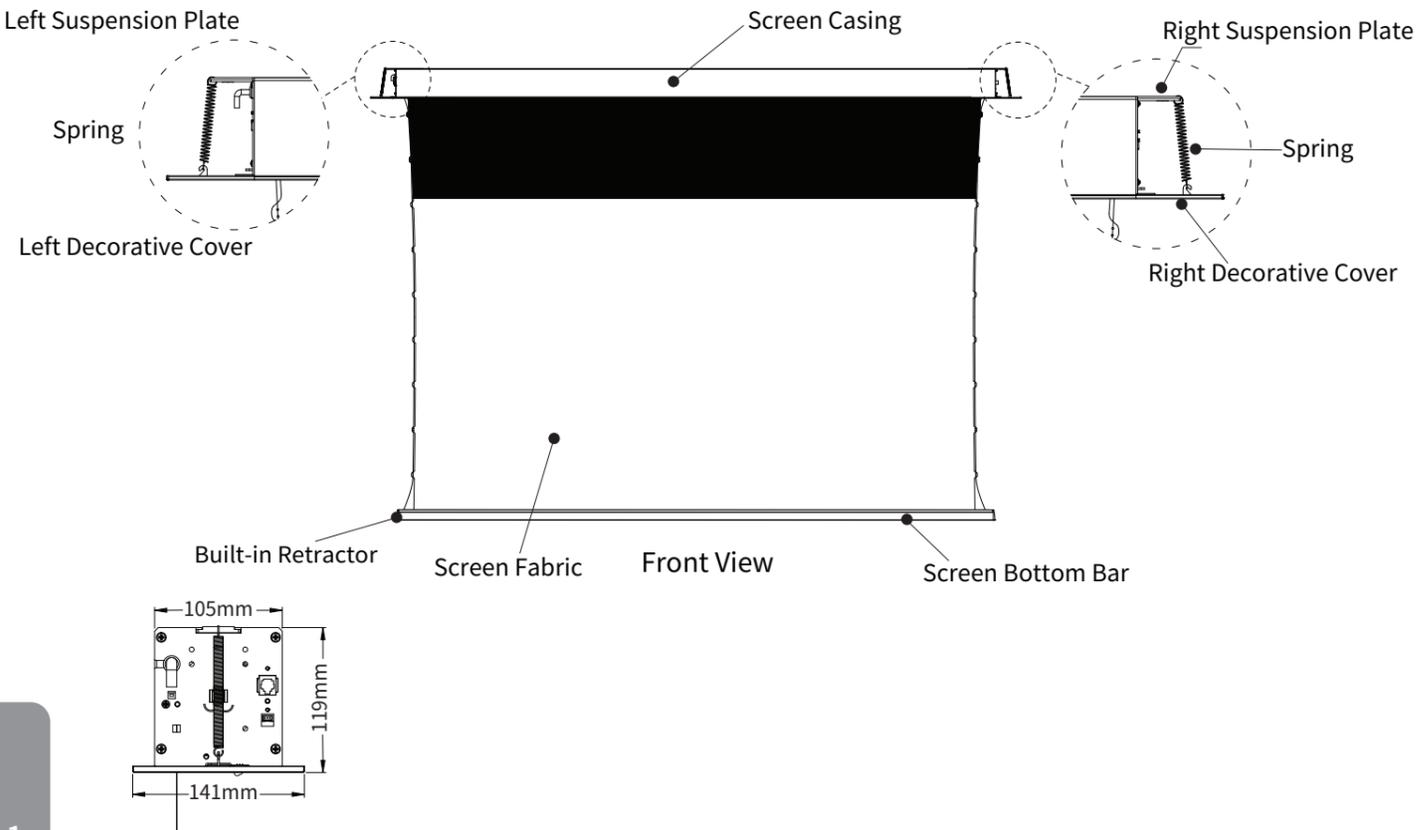
1 Ceiling Opening Dimensions: The length of the opening  $L_t = \text{total length of the screen } L - 25\text{mm}$ , the width of the opening 115mm, height >120mm
