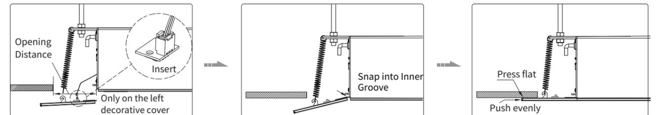
① Before beginning the installation, confirm that the opening has enough clearance. Connect the infrared line, then lightly stretch the spring, and attach it to the decorative cover's hook through the spring's circular opening.
